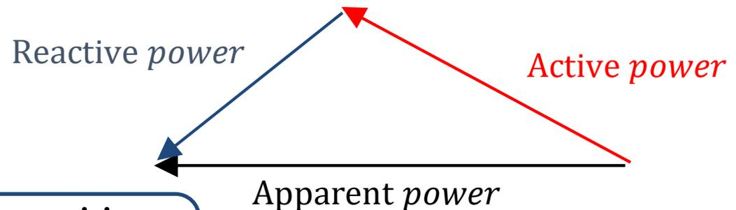
$$\text{PFC} = \frac{\text{Effective power}}{\text{Apparent power}} = \frac{\int \dot{V}i dt}{\bar{V}\bar{I}}$$
